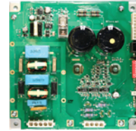
EPC Control Board
